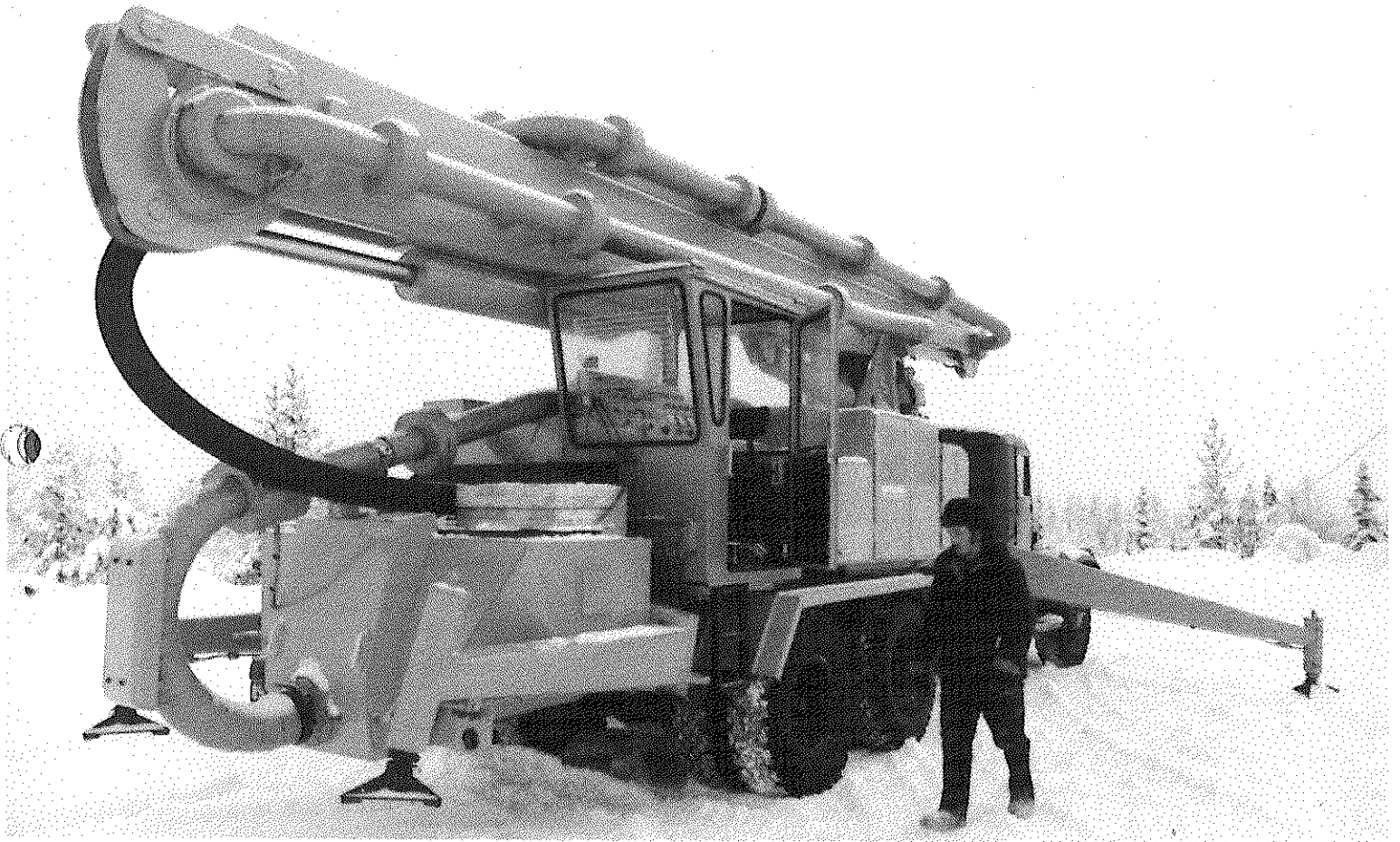
Capable of operating at temperatures as low as -40^{\circ} C, the unique Worthington concrete pump is the result of technological exchanges between Worthington S.p.A. Italy and the USSR.
